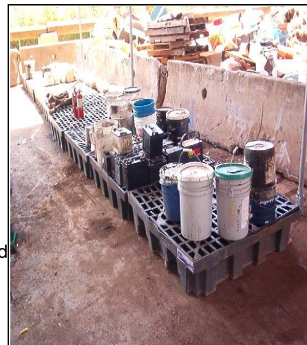
Secondary containment should be used to prevent materials from contaminating stormwater
